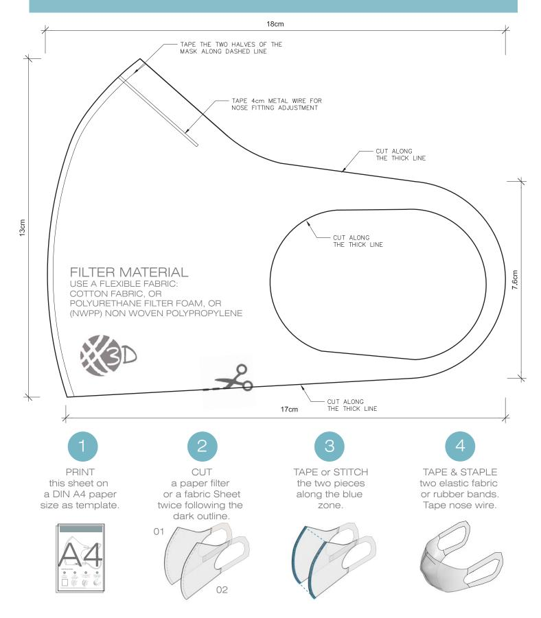
Copyright by DOX3D. Open source facemask geometrical template. Download Tempalte at http://www.dox3d.com/facemask/
